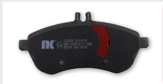
Cut-out of the noise reduction shim
