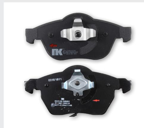
If no arrow is used but the NK pads have a half-moon cut-out in the noise reduction shim, the half-moon needs to be presented at the leading edge where the pad first contacts the brake disc.
